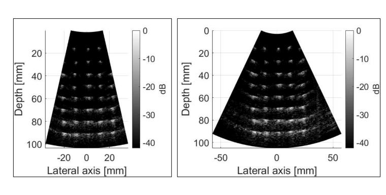
The new images cover a bigger area and are closer to the ultrasound images that doctors have used to see. However, in this approach, a bigger data storage space is needed and the lateral resolution is decreased as a function of the imaging depth, due to the peculiarity of polar coordinates.
