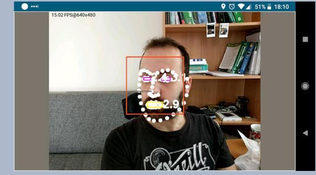
The pose estimation works robustly on a variety of environments, unless scene is too dark and is mostly limited by the face detector.
